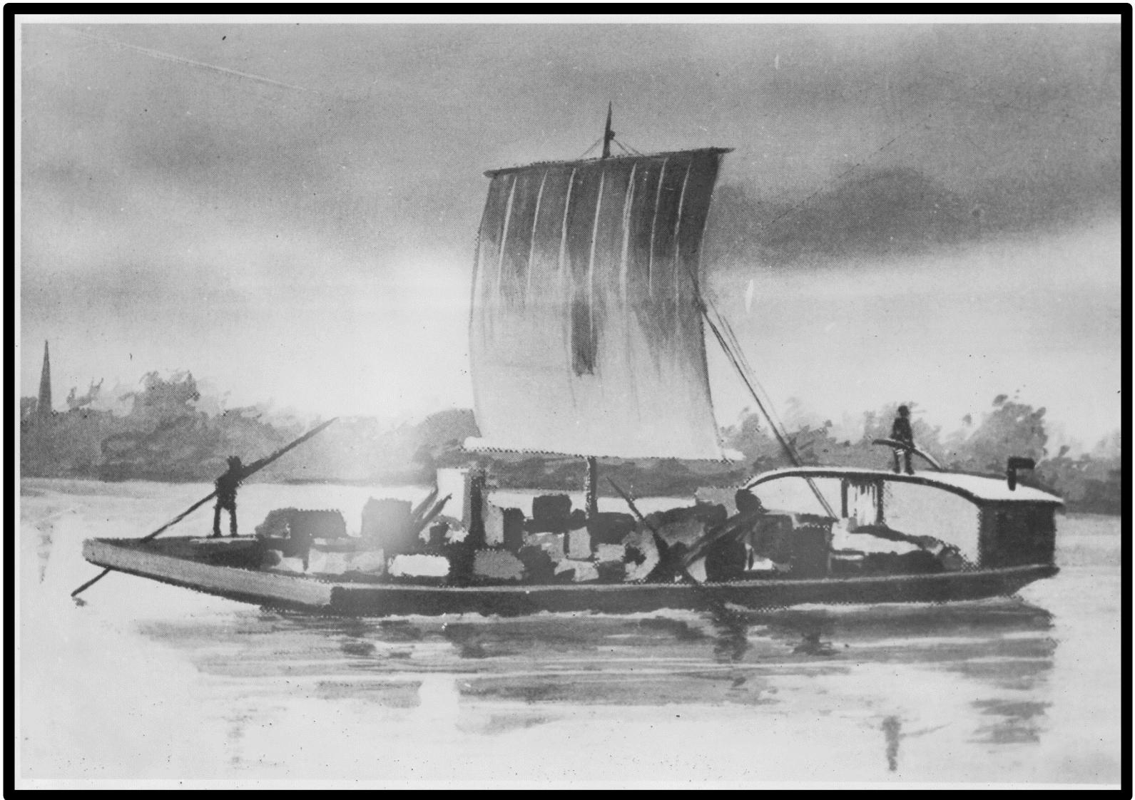
Typical Connecticut River Flat Boat Maximum of 72 Feet Long X 11 Feet Wide; 2 to 3 Ft of Draft; Crew of 7
