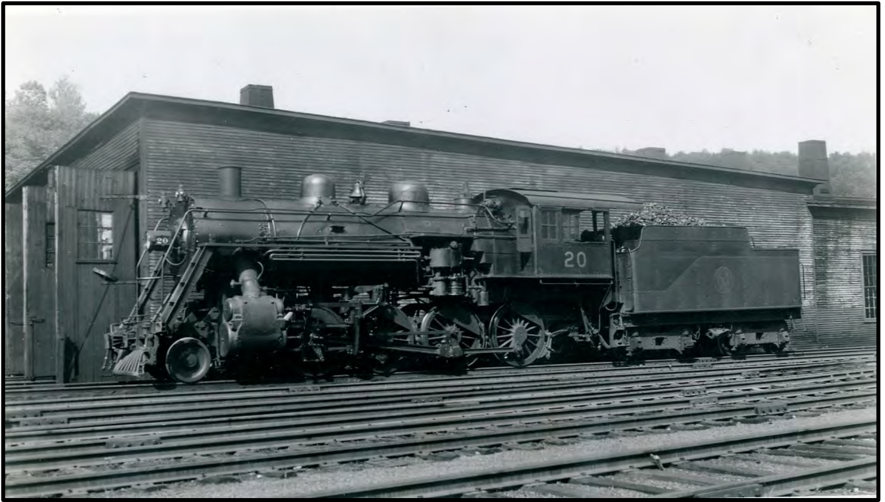
Another view of M&WRR #20 and the Montpelier engine house in the background. These were 2-8-0 "Consolidation" type locomotives designed primarily for freight hauling.
